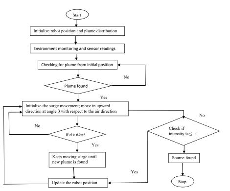
Fig. 1. Flowchart of Casting method for gas leakage source localization by a mobile robot
