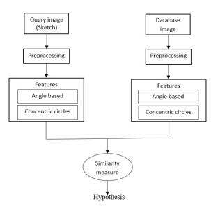
Fig. 1. Propose architecture of Sketch Based Image Retrieval
