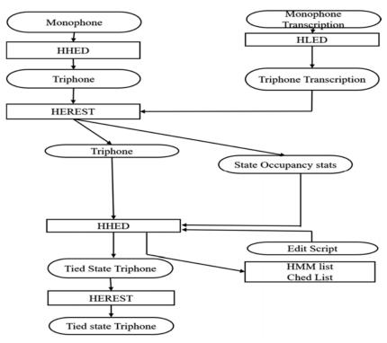
Fig. 1. Triphone based speech recognition system
