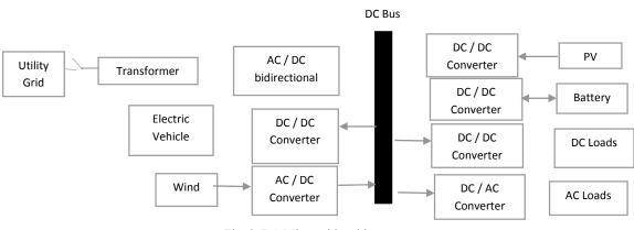
Fig. 3. DC Microgrid architecture
