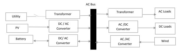
Fig. 2. AC Microgrid architecture
