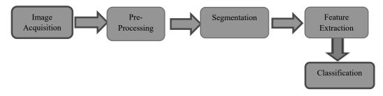
Fig. 1. Lung Image processing system
