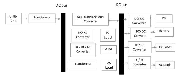
Fig. 4. Hybrid AC/DC Microgrid
