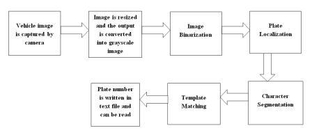
Fig. 2. Block Illustration of Vehicle Number Plate Detection
