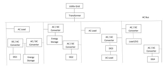
Fig. 1. Architecture of a Microgrid
