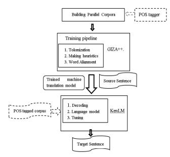
Fig.2. System flow chart of the SMT
